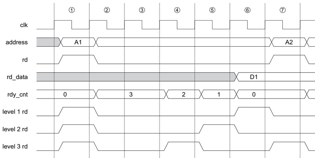
Figure 4: Different pipeline levels for a read transaction
