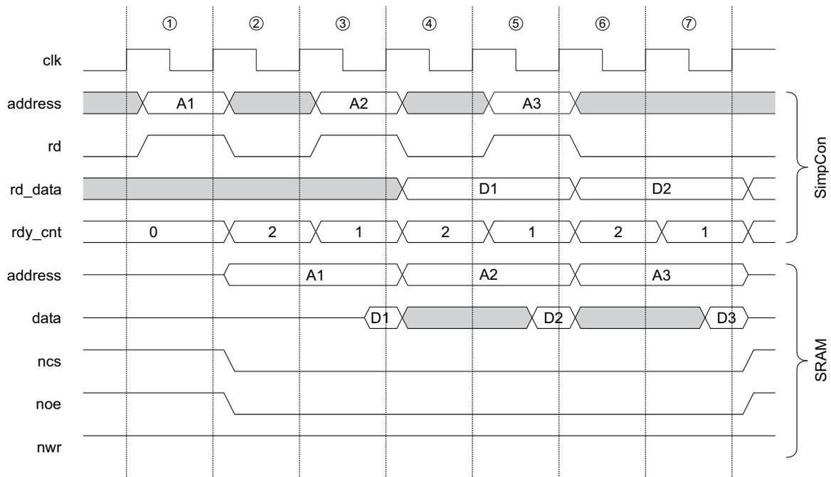
Figure 7: Pipelined read from a static RAM
