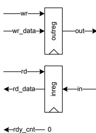
Figure 5: A simple input/output port with a SimpCon interface
